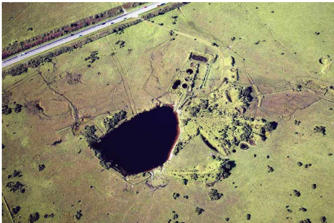
Nineteenth century china clay workings at Burnt Heath, Cardinham. Finger dumps of waste lie to the right of the abandoned pit. Circular and rectangular settling tanks also survive. Photo © Cornwall County Council Historic Environment Service
