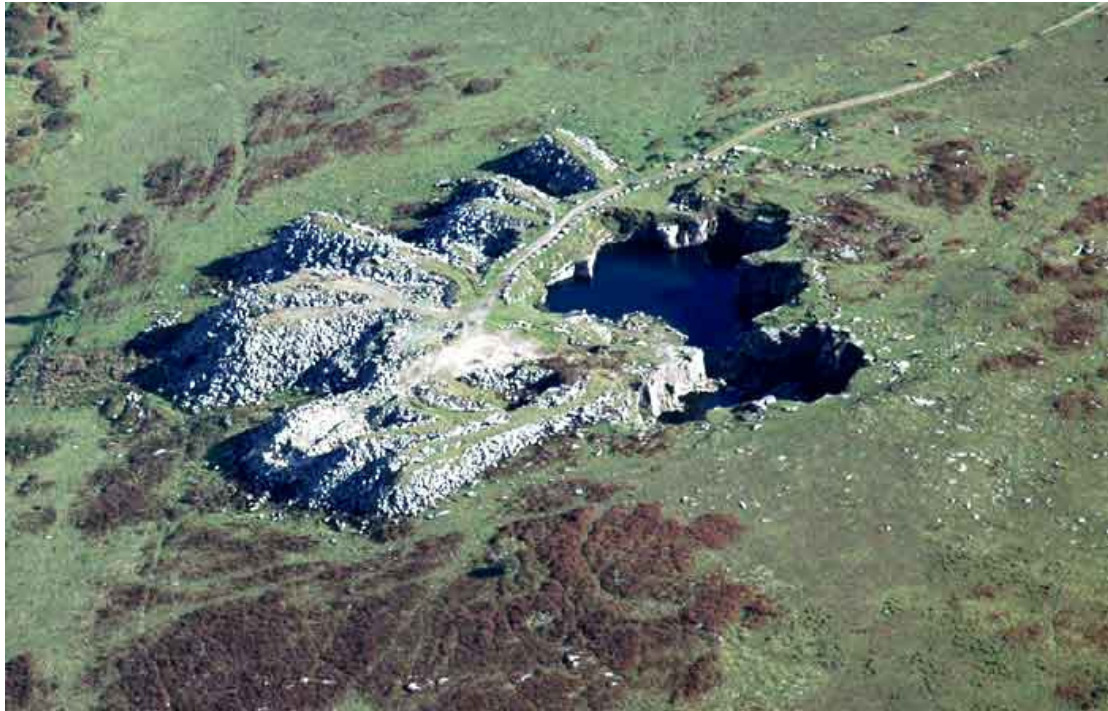
A dimension stone granite quarry at Goldiggings, Bodmin Moor. Dimension quarries are typically steep-sided because the quality of the stone improves the further it is below ground surface. Much of the stone shaping or dressing was done at the quarry. Only high quality, flawless granite could be used so there were large quantities of rejected stone. This was wheeled along tramways to form enormous 'finger dumps' of waste rock which characterise this type of quarry. Photo © Cornwall County Council Historic Environment Service
