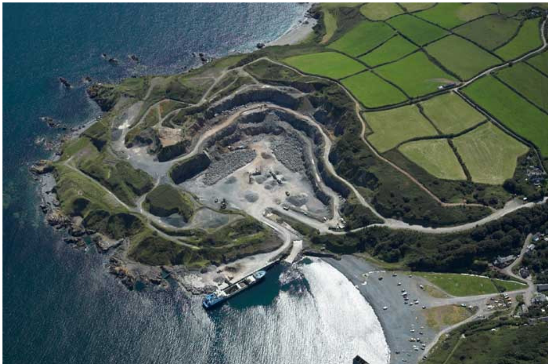
Porthoustock Quarries, St Keverne. Large scale quarrying on the coast of the Lizard Peninsula began in the early 1890s, exploiting gabbro and greenstone for use as aggregates. The crushed rock was carried by tramway to quays on either side of Porthoustock Cove. Fine waste from the quarries and from loading operations at the quays accumulated on the beaches. Beaches in the area have extended seawards by more than 100 metres as a result. Photo © Cornwall County Council Historic Environment Service
