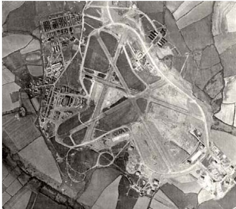
The Naval Air Station at St Merryn, Padstow in 194-. The four runways are designed for short take-offs into the prevailing wind to replicate take-off from aircraft carriers. © English Heritage (NMR): RAF Photography: CPE/UK/1995/1420
