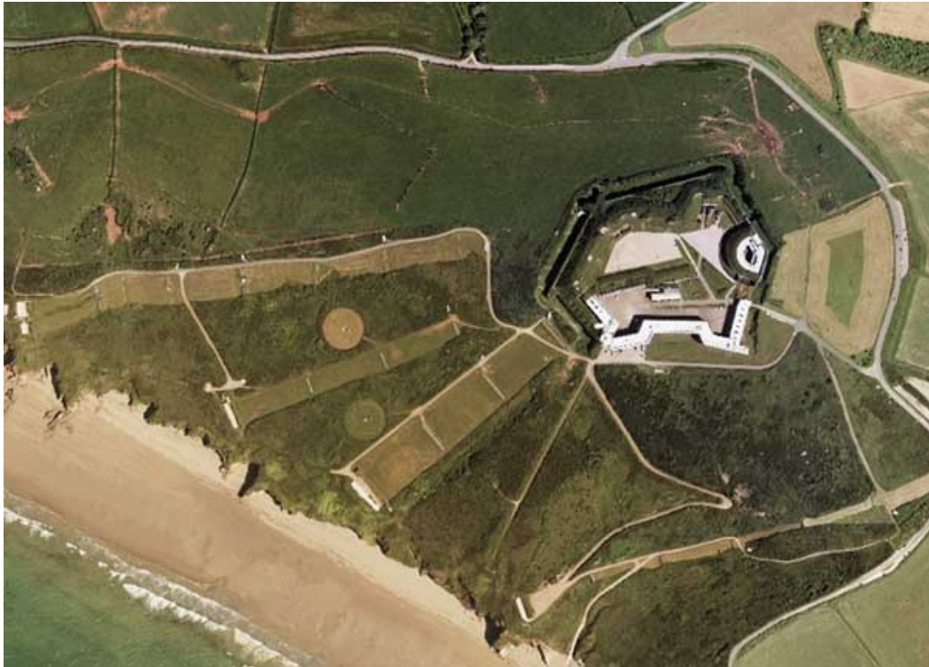
Tregantle Fort. This is the largest land fort in the Plymouth defences and includes a self-contained, ditched keep (to the left). It was built in 1858-59 to house 2,000 men in barracks arranged on its south side (facing the camera in this view) and was designed for 35 guns. Photo © Cornwall County Council Historic Environment Service
