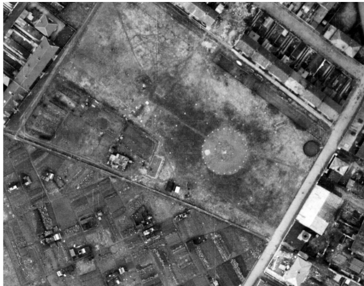
The base for a barrage balloon at Torpoint. The small white dots that form concentric circles are the remains of concrete blocks set into the ground and used to anchor the balloon's mooring cables. © English Heritage (NMR) RAF Photography: 106G/UK/1274/5083
