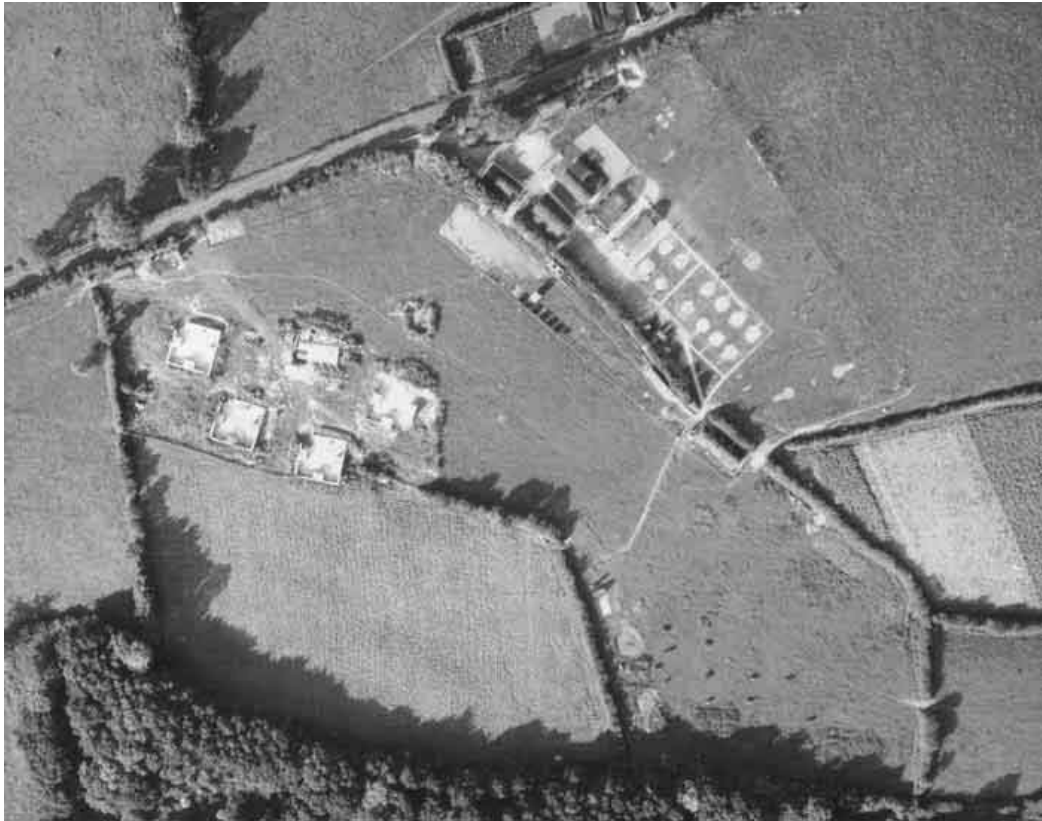
Remains of a heavy anti-aircraft battery. This shows the typical layout of four 3.7 inch gun emplacements arranged in a horse-shoe layout with the command centre set slightly back. © English Heritage (NMR) RAF Photography
