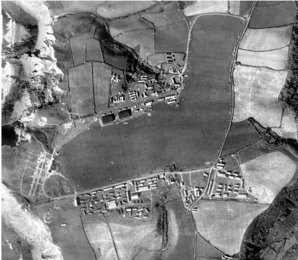
The anti-aircraft gunnery range at RAF Cleave near Bude, showing the grass airfield, the gun batteries on the clifftop (to the left) and the circular base for the steam catapult launcher (just below the gun batteries). © English Heritage (NMR) RAF Photography: CPE/UK/1793/3045
