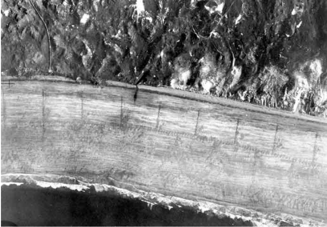
The site of beach scaffolding at Hayle Towans. Defences such as these were in use for only a few years before being dismantled and have left little trace. At Hayle the scaffolding posts have left an imprint forming a line parallel with the coastline; the supporting steel struts have left lines at right angles to this. © English Heritage (NMR) RAF Photography: S747/6009
