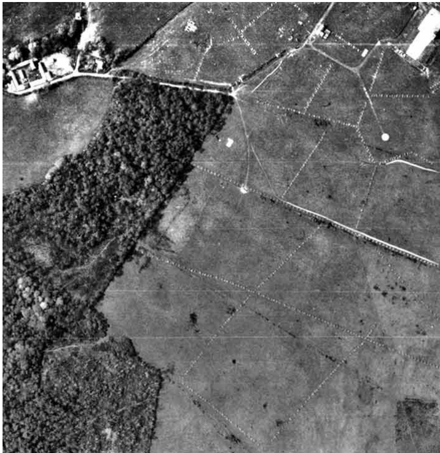
Aircraft obstruction pits at the site of the 1914-1918 war airship base at Bonython on the Lizard Peninsula. Much of the surrounding area, in the vicinity of Predannack airfield, was considered vulnerable to airborne landing of invasion troops and was criss-crossed by rows of these pits. © English Heritage (NMR) RAF Photography: 3G/TUD/UK/211/5224
